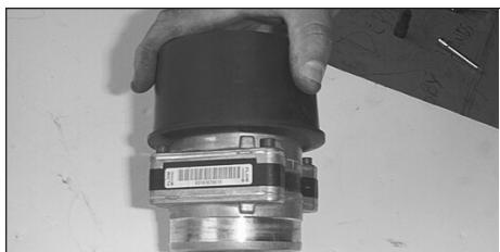
21. Install the filter adapter onto the mass air sensor with the directional arrow as shown above.
