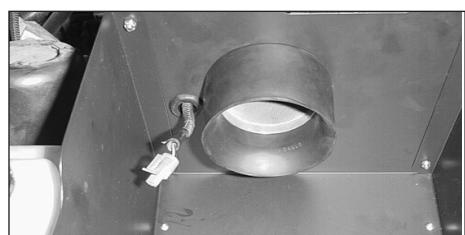
25. Install the factory air temperature sensor lead through the grommet hole on the heat shield.
