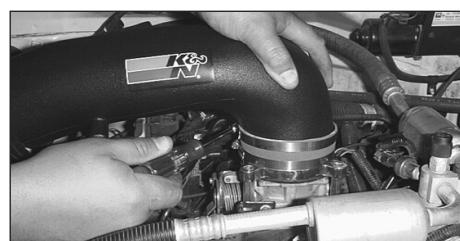
29. On models with air injection, attach the air injection hose to the flange on the vent filter using the O.E. clamp.
