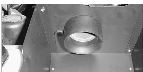
22. Install the mass air sensor into the hole on the heat shield as shown.
