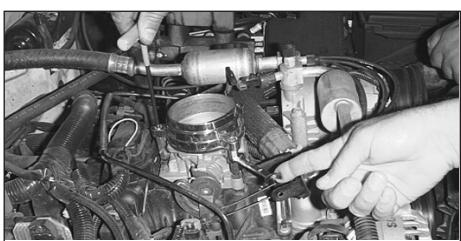
17. Using a 7/16" wrench, snug the three coupling nuts and tighten the three 6mm bolts using a 5mm allen wrench.
