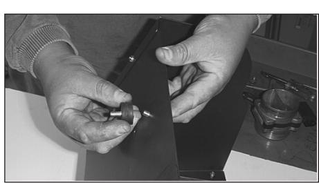
20. Using the provided hardware, install the rubber mounted studs onto the bottom side of the heat shield.
