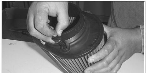
24. Reinstall the factory air temperature sensor into the provided hole on Filtercharger element.
