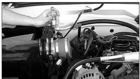
27. Install the mass air adapter onto the mass air sensor and tighten mass air sensor side only.
