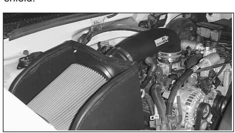
26. Place the filtercharger element into the heat shield and reconnect the air temperature sensor electrical connection, then slide the element onto adapter and tighten with provided hose clamp.
