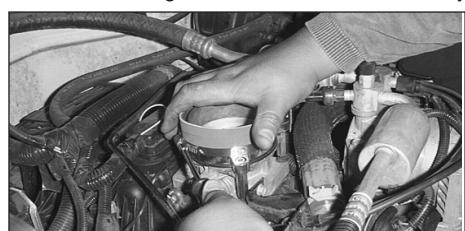
28. Install the silicone hose over the throttle body adapter and tighten using a provided midi hose clamp.
