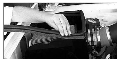
32. Install trim seal onto the heat shield. **NOTE:** Some cutting and trimming may be necessary to achieve best fit.
