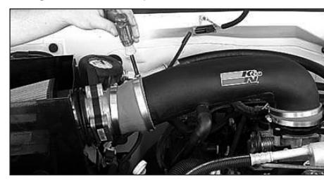
30. Fully install the K&N intake tube onto the throttle body adapter and tighten second midi hose clamp.
