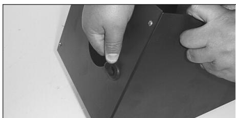
19. Install the provided grommet into the small hole on the heat shield.
