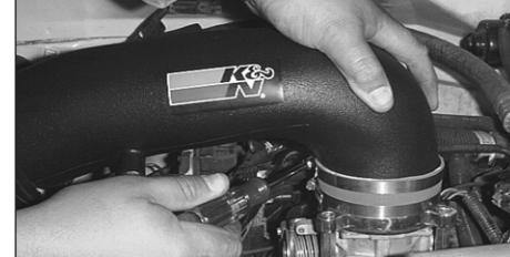
31. Reconnect the crankcase vent hose onto the intake tube.
