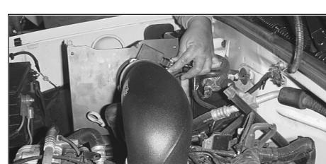
33. Reconnect the mass air sensor electrical connection.
