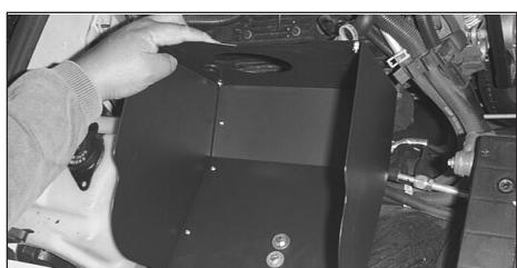
23. Install the heat shield assembly into the two holes on the inner fender and secure from underneath. **NOTE:** Apply the poron gasket onto the heatshield to cover the exposed bolts.
